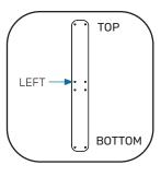
The distro plate must be mounted on the left-hand side. The mounting holes on the back can be used for this, as shown in the illustration.
