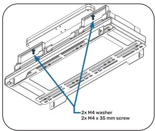
The distro plate can be flexibly moved up or down on the mounting bracket.
