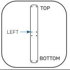
The distro plate must be mounted on the left-hand side. The mounting holes on the back can be used for this, as shown in the illustration.
