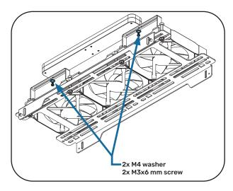
The distro plate can be flexibly moved up or down on the holder.
