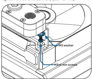
Do not overtighten the screws to avoid cracks in the acrylic glass.
